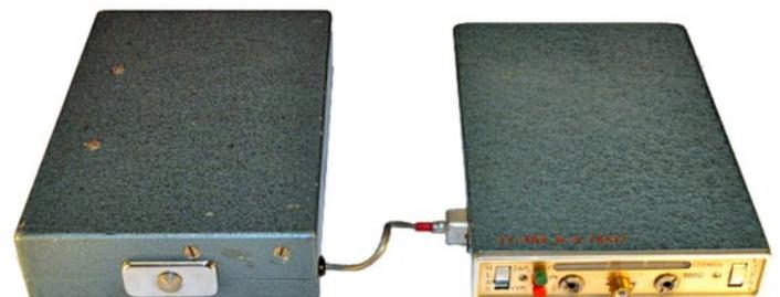
A separate power unit, comprising two 4.5V flashlight batteries (left), or a AC mains power supply connected to the Sázava III receiver.
