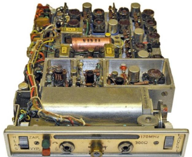
View of front panel and general components layout of the Sázava III.
