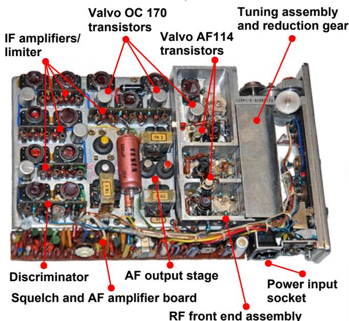
Top view the Sázava III assembly with functions of the various modules and components.
